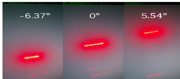
Fig. 7 Representative laser scanning traces generated by the scanning mirror with the fast and slow axes driven at 206 Hz (fast) and DC (slow) in water.
