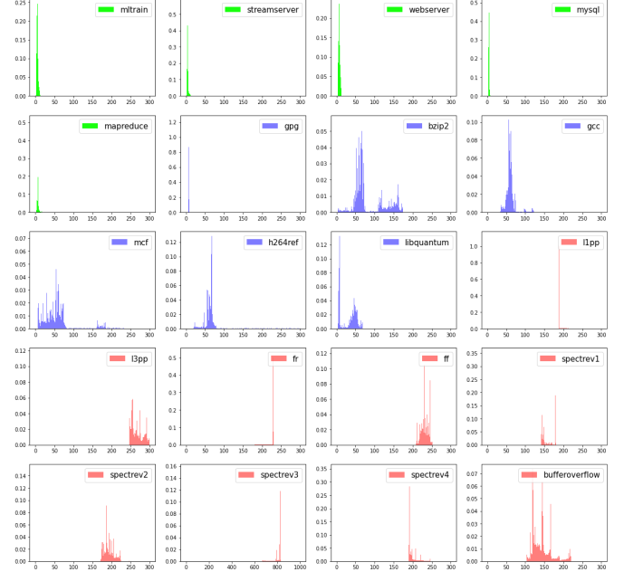
Fig. 3: Reconstruction error distribution (RED) of normal cloud workloads (first five in green), benign programs (next six in blue) and attacks (last nine in red). RED of all attacks are different from the normal behavior of the cloud workload. The x-axis is the magnitude of RED, and y-axis is the probability density of that RED magnitude.
