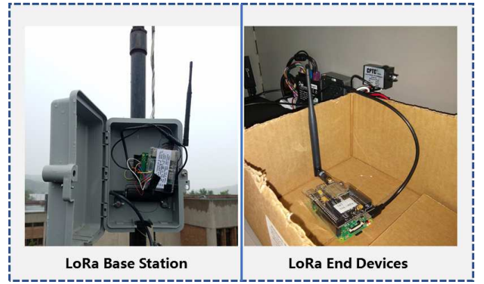
Fig. 3. Hardware deployment for our LoRa network.
