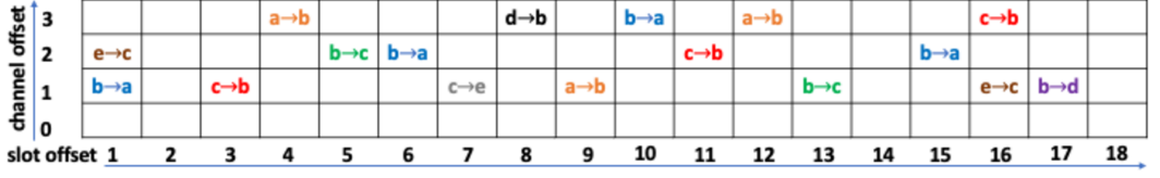
Fig. 9. Example cell allocations to four pairs of bidirectional links in Figure 1(a). A slotframe that consists of 18 slots is divided into eight subslotframes.
