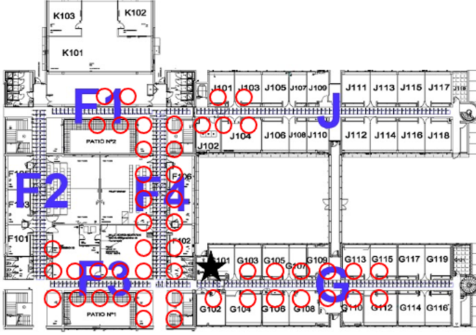
Fig. 2. Testbed used for our studies. All 50 devices are deployed on the same floor in an office building. The black star indicates the device that serves as the border router (Root) and the red circles denote end devices.
