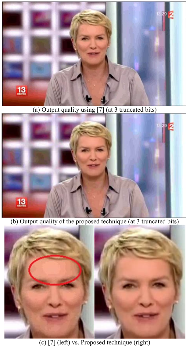
FIGURE 2. Observer discernable flaws in the facial region due to a “banding effect” on the face when comparing (a) and (b) caused the overall quality of the frame to become unacceptable at 3 truncated bits (Video tag: wF6lvdXXwc4 from [14]).
