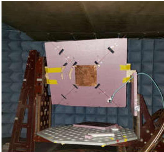
FIGURE 10. Experimental setup showing the realized UAV model inside the GTEM and the current probe at one location.
