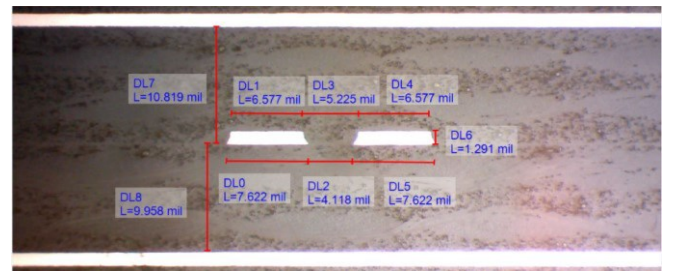
Fig. 11. Cross section of the coupled striplines.
