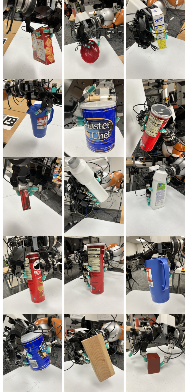
Fig. 4: Example precision grasps resulting from our controller.
