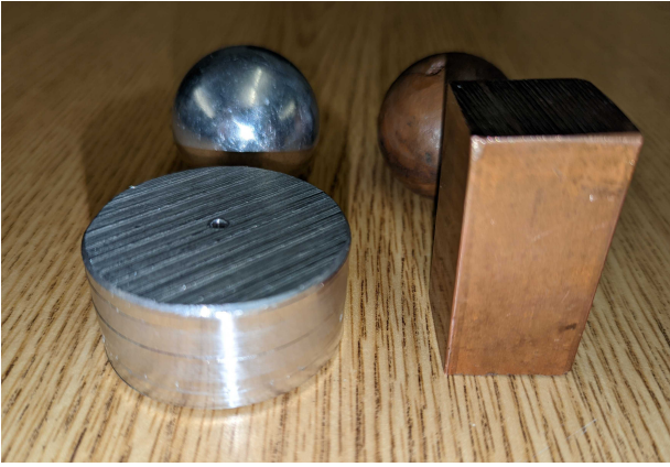
Fig. 5: The four objects used in our manipulation experiments: (back, left) a solid aluminum sphere of radius 20.0 mm, (back, right) a solid copper sphere that we approximate as having a radius of 20 mm but by mass-density has an effective radius of 19.8 mm, (front, left) a piece of aluminum scrap approximately cylindrical in shape with radius 25.2 mm and length of 23.1 mm with a hole in the center that is counterbored from one side, and (front, right) a solid, elongated copper cuboid with length 50 mm cut from a 25.4 mm square stock.
