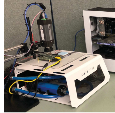
Figure 1: IR thermography setup used to collect training data in this work
