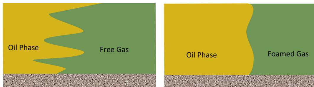
Figure 14. Schematic of gas flooding (left) vs foam flooding (right). Foam flooding reduces viscous fingering by modifying the mobility ratio. Schematic was drawn with the idea from ref 181.
