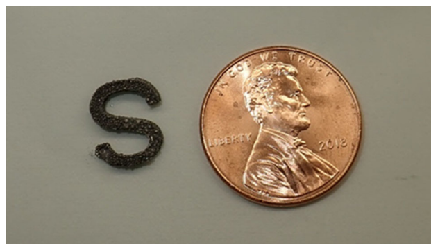
Fig. 7 An “S” shape part made of \text{Bi}_2\text{Te}_3 is made additively using laser powder bed fusion. The thickness of the specimen is greater than 1 mm
