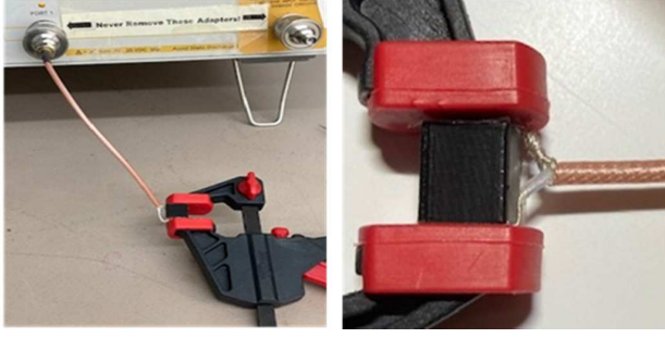
Fig. 1. (Left) An image of the parallel plate capacitor connected to the VNA via a coaxial cable and mechanical clamping. (Right) An image of the mechanical clamping used in this measurement. The red blocks are the jaws of the clamp, the black cube is the printed CF20 sample, and the silver wires are the center conductor and shield of the coaxial cable used to connect the parallel plate capacitor to the VNA for measurement.
