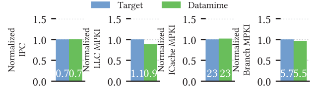
Figure 12: Key performance metrics of Datamime relative to Target for mem-fb with the server and client configured to communicate over the network.
