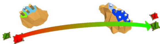
Fig. 4. Software components can be displayed using the “software island” metaphor, showing components and their inter-dependencies. [44]
