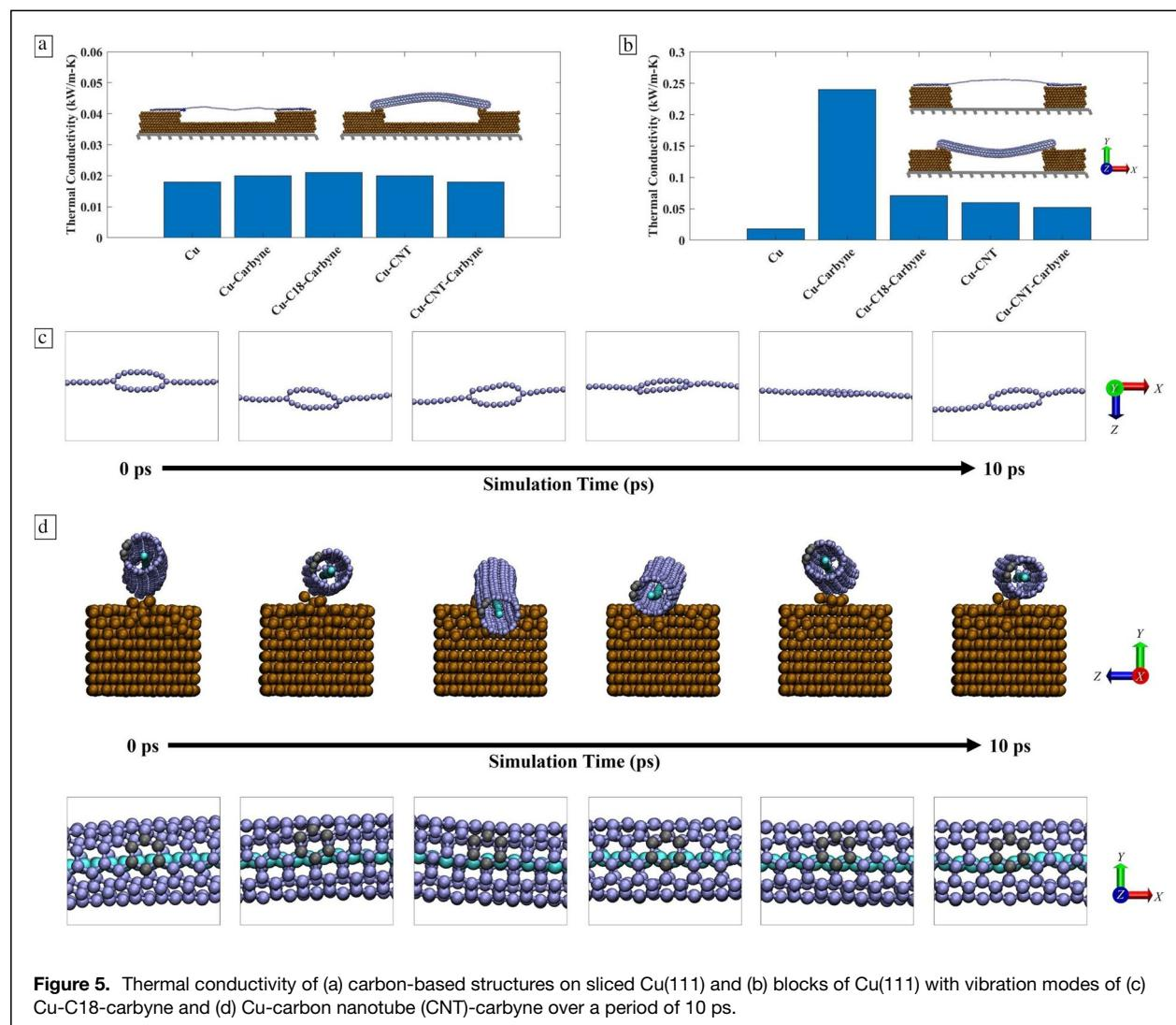
**Figure 5.** Thermal conductivity of (a) carbon-based structures on sliced Cu(111) and (b) blocks of Cu(111) with vibration modes of (c) Cu-C18-carbene and (d) Cu-carbon nanotube (CNT)-carbene over a period of 10 ps.
