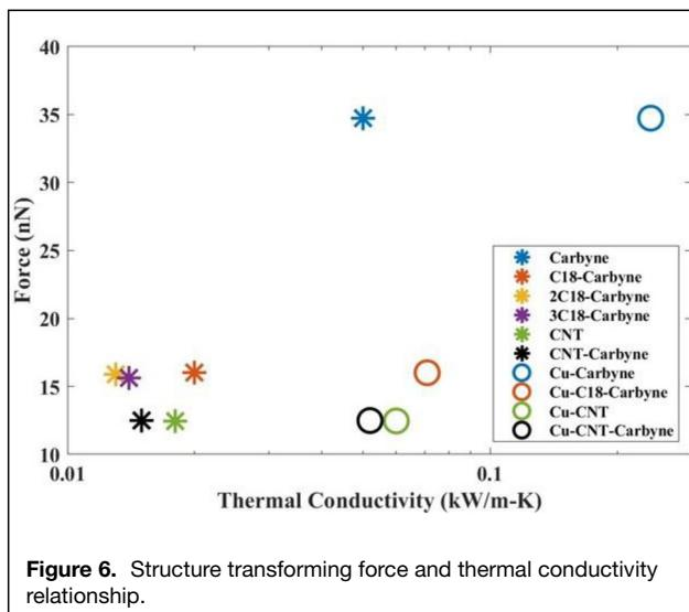
**Figure 6.** Structure transforming force and thermal conductivity relationship.
