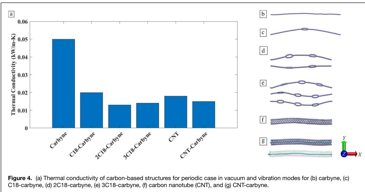
**Figure 4.** (a) Thermal conductivity of carbon-based structures for periodic case in vacuum and vibration modes for (b) carbyne, (c) C18-carbyne, (d) 2C18-carbyne, (e) 3C18-carbyne, (f) carbon nanotube (CNT), and (g) CNT-carbyne.
