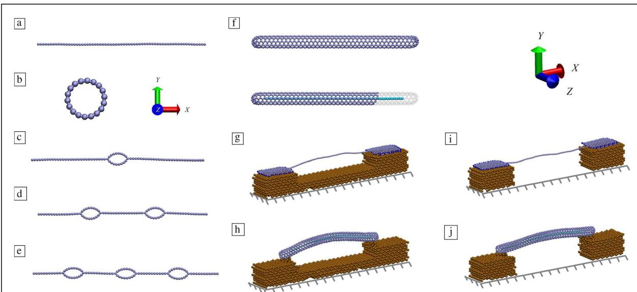
**Figure 1.** Samples used in this study, (a) periodic carbyne, (b) C18 ring, (c) periodic C18-carbyne, (d) periodic 2C18-carbyne, (e) periodic 3C18-carbyne, (f) capped carbon nanotube (CNT), (g) graphene-carbyne on sliced Cu(111), (h) capped CNT-carbyne on sliced Cu(111), (i) graphene-carbyne on Cu(111) blocks, and (j) capped CNT-carbyne on Cu(111) blocks.
