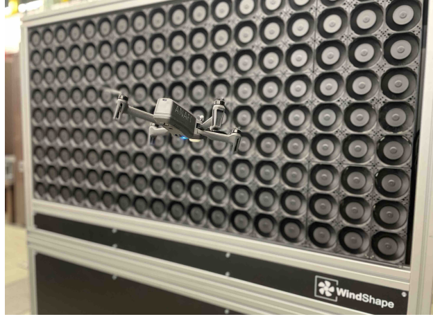
Fig. 3 Parrot Anafi in free flight test in a WindShape testing facility. WindShape, Switzerland, November 2021.
