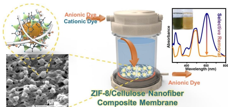
Figure 9. A 21 wt.% ZIF-8 loaded 2,2,6,6-tetramethylpiperidine 1-oxyl radical oxidized cellulose nanofibers membrane. Adapted with permission from Song et al. [279]. Copyright (2019) Elsevier.
