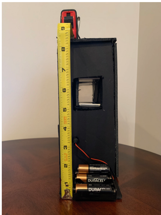
Figure 4. Experimental prototype of the Pepper Ghost Tunnel using cardboard to enclose the transparency film and the two opposed LCDs. The total size of the prototype is 101.6×241.3×190.5mm (Width×Height×Depth).
