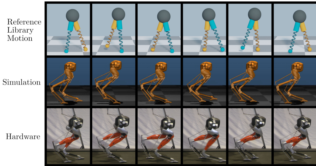
Fig. 8. Motion comparison of the reduced-order model, simulation, and hardware at different phases in the gait. The top images represent the desired reference motion to recreate, the middle images show the learned policy in simulation, and the bottom images show the learned policy executed on hardware.
