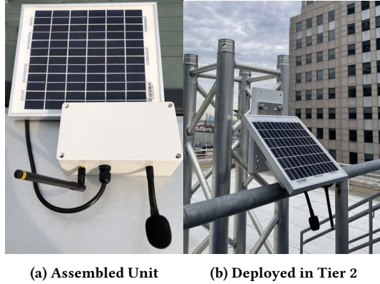
Figure 6: The SONYC MKII device, shown in enclosed form, is affixed behind the solar panel, which is angularly mounted to maximize solar exposure
