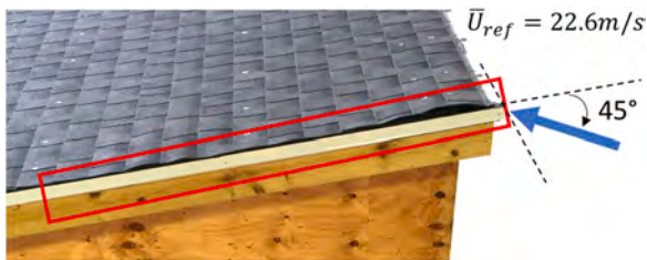
Fig. 22. Shingle liftoff before edge nails.
