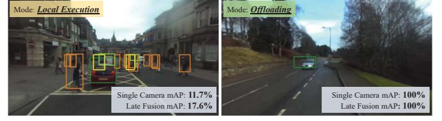
Figure 2: Two frames of different complexities showing single camera and late fusion mAP scores and the selected operational modes by our learning-based solution. The bounding boxes indicate the ground truths from the dataset.
