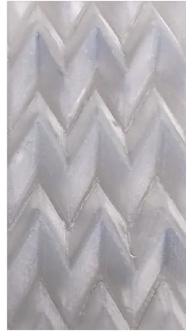
Figure 4: Photographs of each Miura-patterned capacitor design with a 3\times 3 cell view of the A, B, and C patterns after fabrication. The scale is constant across these photographs.
