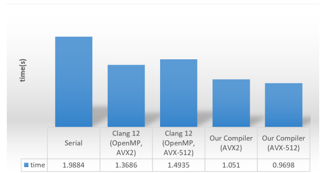
(a) Runtime (seconds) for Sparse Matrix-Vector Multiplication: on Intel 6230N for AVX2 (256-bit vector length) and AVX-512 (512-bit vector length)
