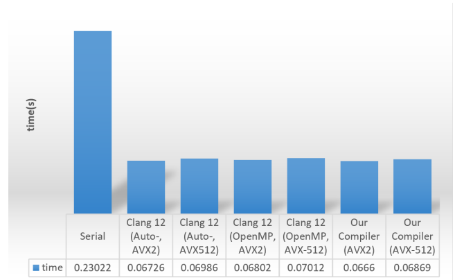
(a) Runtime (seconds) for AXPY: on Intel 6230N for AVX2 (256-bit vector length) and AVX-512 (512-bit vector length)
