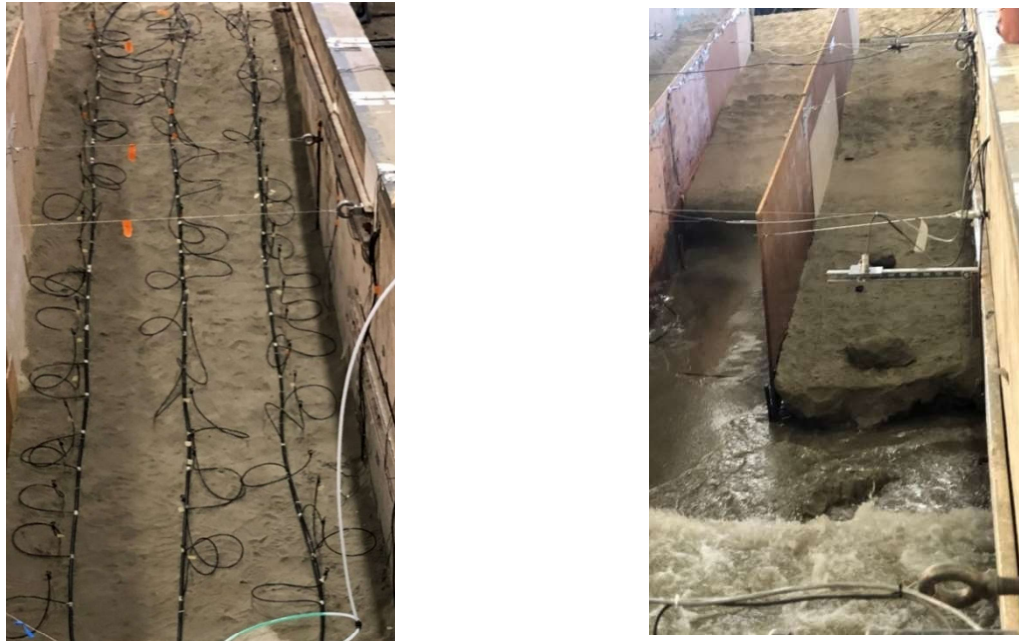
Figure 3. Surface spraying setup and used for the second dune (left); treated and untreated zones during testing (right).
