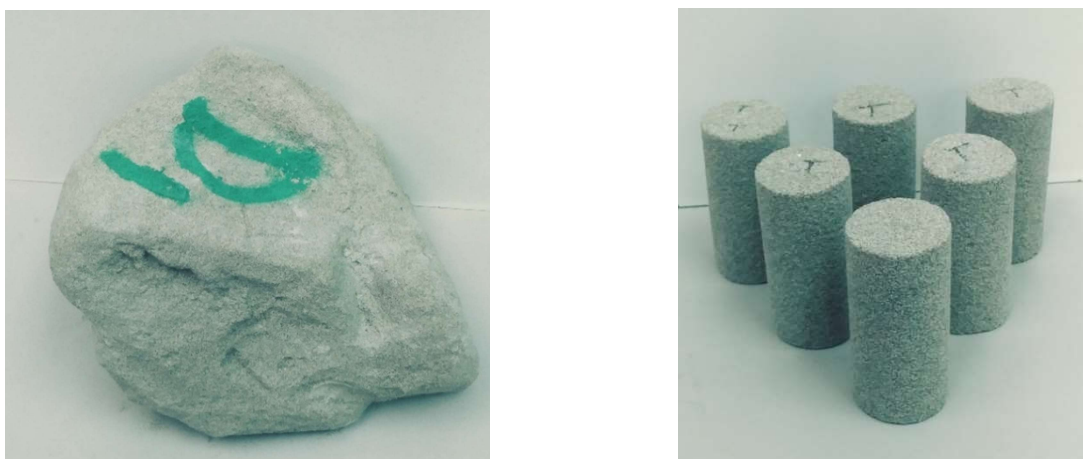
Figure 5. A bio-cemented chunk from the treated surface (left) and prepared specimens for triaxial tests (right).
