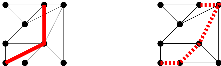
Figure 7: (Left) An underlying network and a path of two edges from the overlay network on top of it. (Right) The overlay network path will be automatically resolved into a path of physical links in the base graph, by resolving each edge into a shortest path between its endpoints.
