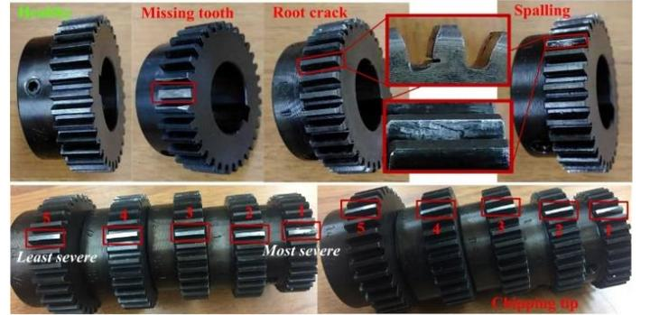
Figure 2. Fault conditions.
