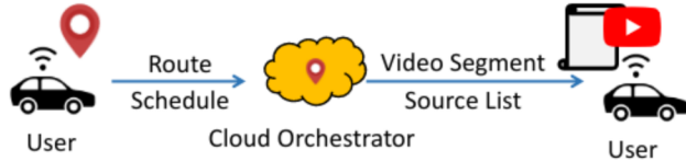
Figure 7: The cloud orchestrator analyzes the user's route information and produces a video segment source-list for the user. This list contains information about the edge nodes the user can obtain content from as it travels through the declared route.
