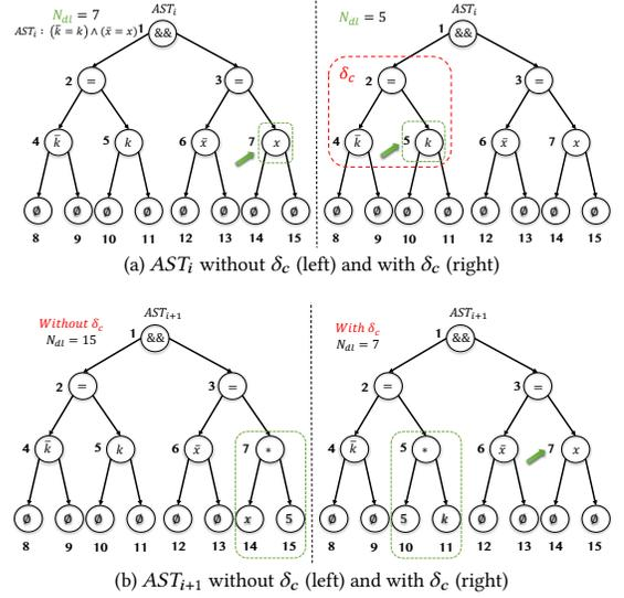
Figure 3: Constructing the next AST by modifying the current AST. The  $i$ -th candidate shown in (a), with and without the conflict predicate  $\delta_c$ . The  $(i + 1)$ -th candidate shown in (b), with and without  $\delta_c$ -based pruning.
