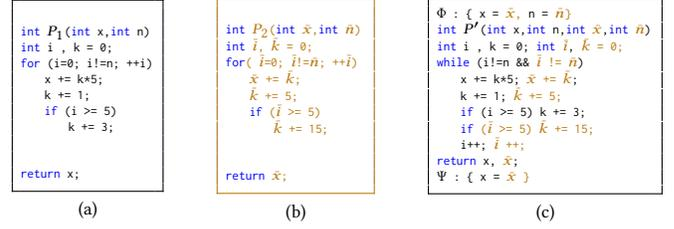
Figure 2: Given two programs  $P_1$  and  $P_2$ , we merge them into a single program  $P$  to execute the instructions in lockstep.
