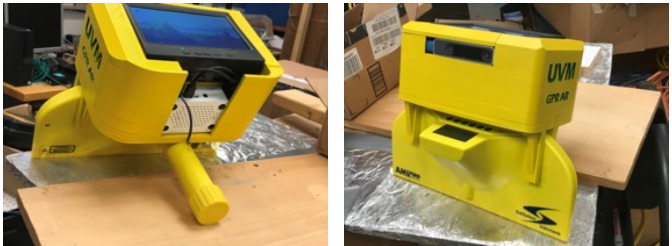
Figure 1. The AML Pro CW radar is shown here with the attached 3-D printed enclosure for the Raspberry Pi 4, Intel Realsense T265 along with all necessary batteries and an HD screen for user interface
