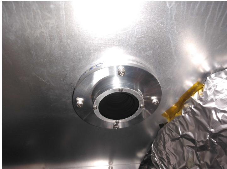
Figure 12. Position and schematic cut view of the baffle tube assembly (left) and an image of the baffle tube mounted on the inner wall of the MYSTIC cryostat (right). The baffle tube consists of a series of varying inner-diameter traps coated in Singularity Black paint, which absorb stray thermal background light.
