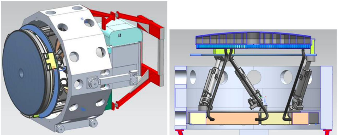
Figure 11: Left: concept for an ASM for Keck housed in an existing Keck top-end hexagonal structure that defines at the secondary socket. Right: cross section showing the ASM mounted on a hexapod for precision static alignment.
