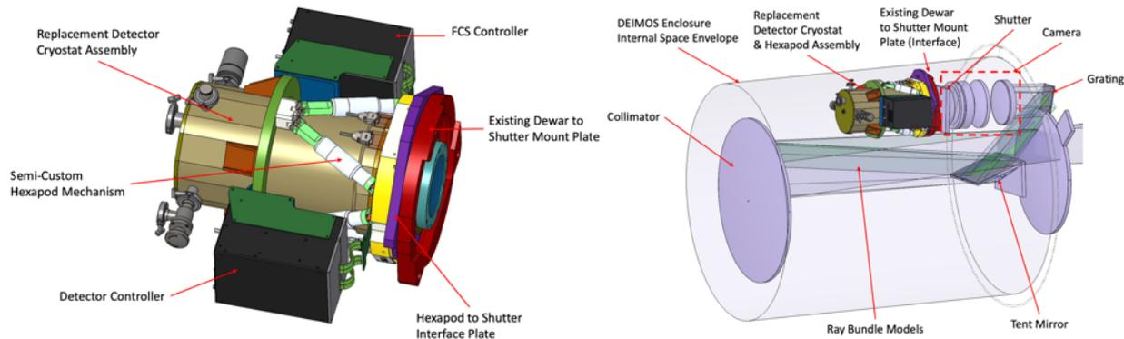
Figure 10: Left: Rendering of the DEIMOS upgrade subcomponents. Right: The shutter mount plate is the interface with the existing spectrograph and the upgrade components are show in context with the DEIMOS optical layout in the instrument barrel.
