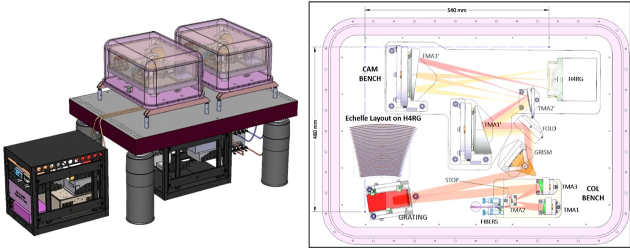
Figure 7 Left: HISPEC instrument layout including 6-foot lab bench, electronics racks, and cryostat to be in the basement of Keck II. Right: Top view of the spectrograph opto-mechanical layout inside the cryostat.
