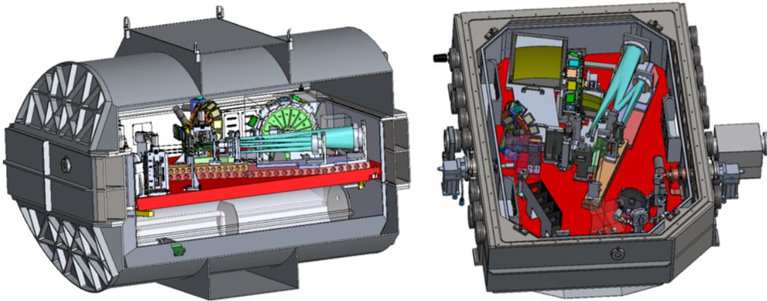
Figure 8 SCALES cryostat and opto-mechanical layout as presented during a preliminary design review. The optical bench is a single layer with two detector systems for both an imager and IFS. SCALES rides on a cart that can roll into the KII AO enclosure.
