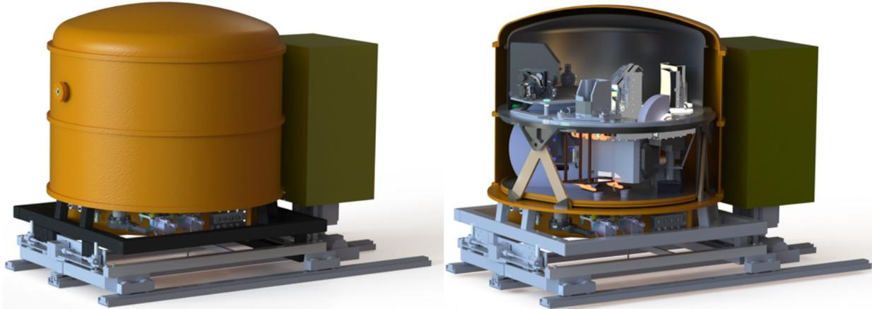
Figure 9: (Left) Liger cryostat on the transfer cart with entrance window on the cryostat. (Right) Cross section of the cryostat revealing the subsystem layout above and below the primary optics bench.
