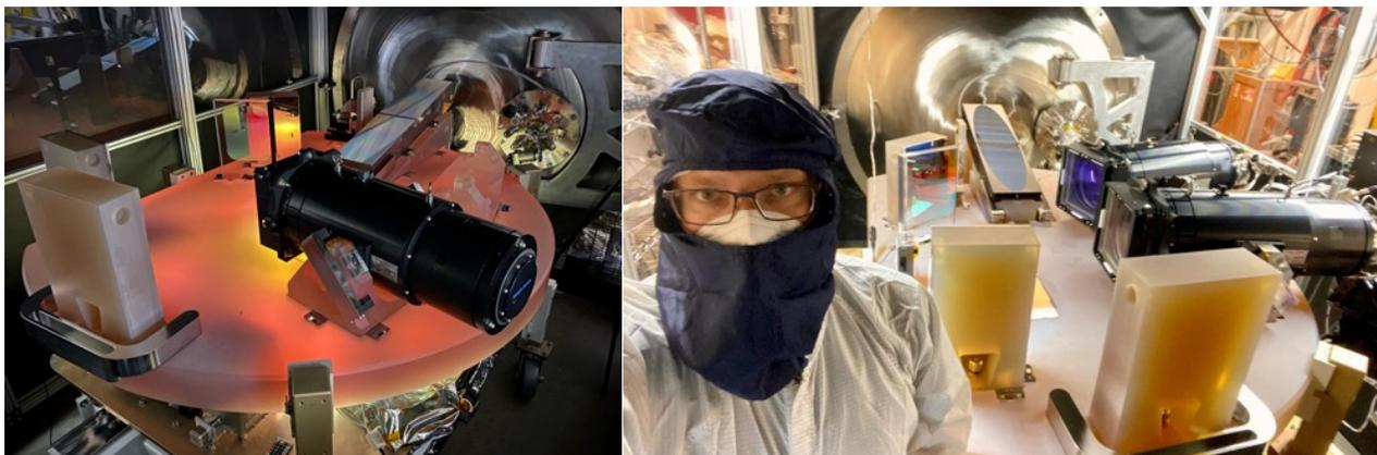
Figure 4 Left: Keck Planet Finder illuminated from underneath showing subsystems delivered during AIT in November 2022 by Jerry Edelstein. Right: PI Andrew Howard next to the fully populated optics bench and vacuum chamber May 2022.
