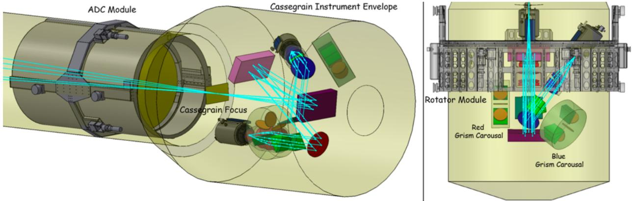
Figure 12: Conceptual optical layout for LRIS-2 with the volume of the KI Cassegrain socket defining the instrument envelope. Also depicted is the existing ADC module that LRIS II will reuse. Top-down view of the instrument with a facility rotator module.
