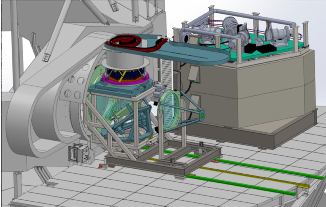
Figure 13: FOBOS conceptual layout on the KII Nasmyth Deck. The forward module that houses the ADC, guiding system, calibration system, and Starbugs fiber positioners. The layered bank of spectrographs has four optical channels and is will be a permanent installation on the Nasmyth deck.
