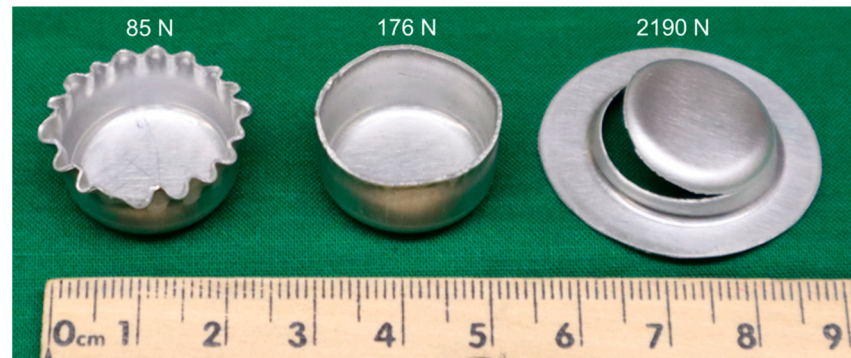
Figure 1. Aluminum AA1100-O cups drawn under different BHF (from left to right: wrinkled (low BHF), fully drawn (medium BHF) and torn (high BHF)). The numbers listed are the BHF.
