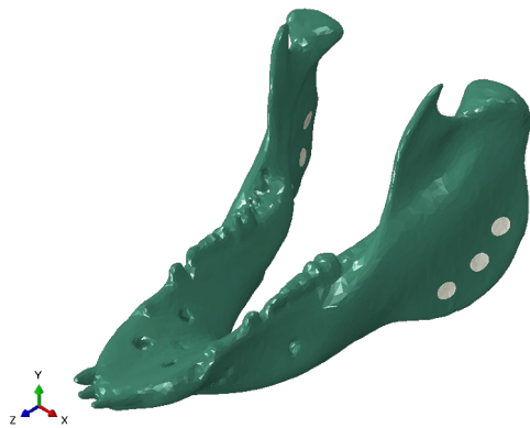
FIGURE 6: Isometric view of the mandible geometry. The scaffold regions are shown in grey.
