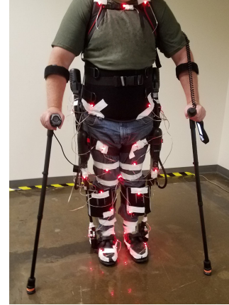
Fig. 1. EksoGT operator using Lofstrand crutches
