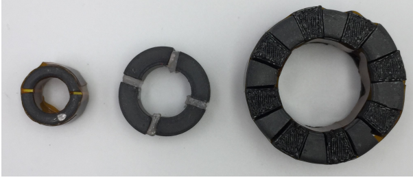
Fig. 5: Unwound toroidal cores showing implementation of quasi-distributed gaps for 10, 30, and 60 MHz.
