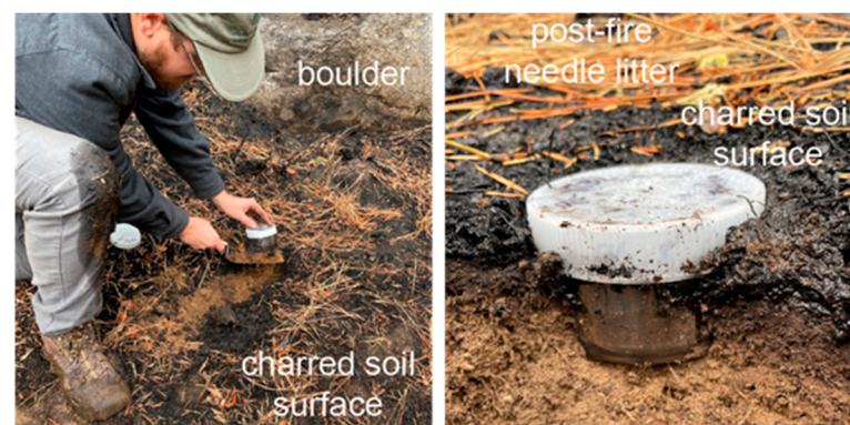
Figure 2. (Left) Collection of core samples for measuring soil hydraulic and thermal properties. Samples were carefully excavated to minimize sample disturbance. (Right) Close-up view of core sample in place prior to excavation.
