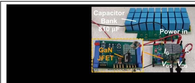
Fig. 3. (a) Schematic of the SC test circuit. (b) Schematic of the RC interface gate driving circuit with all component values marked. (c) Photo of the test setup.
