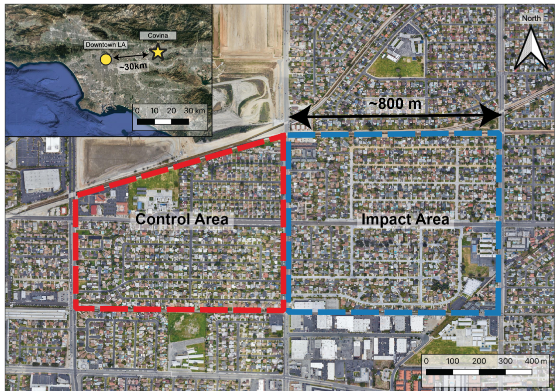
Figure 1. Map of the measurement site in Covina, CA. The impact area (with cool pavements) is shown in blue, while the control area (without cool pavements) is shown in red. The inset map in the upper-left corner shows the Covina site with respect to downtown LA and the greater LA metropolitan area. Map data ©2020 Google.
