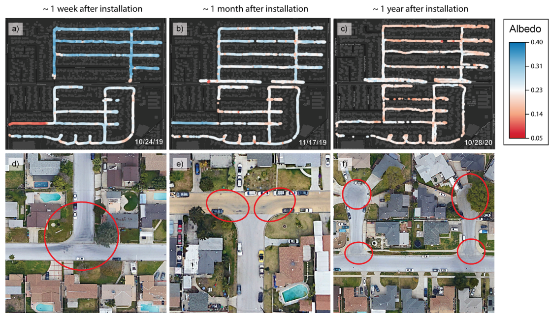
Figure 6. Panels (a)–(c) show a ‘heat-map’ of albedo ~1 week, ~1 month, and ~1 year after cool pavement installation, respectively. Panels (d)–(f) show satellite imagery of representative areas of cool pavement with marked albedo decrease (highlighting with red circles) in the impact area. Map data ©2020 Google. © OpenStreetMap contributors.
