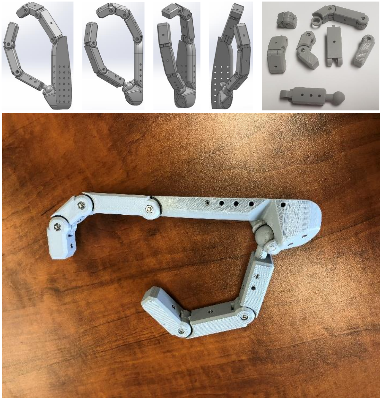
Figure 17. Top: CAD Modeling and components of the finger pieces. Bottom: Fully assembled 3D-printed human-like hand scaffolding with low friction joints and threaded heatsets for the EAP attachment areas, biomimetically designed around the first and second digits (partial hand for first iteration on pincer grip).
