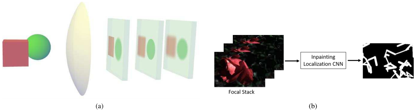
Fig. 1: Focal stack system for inpainting region localization. (a) Imaging system schematic showing depth dependent defocus blur of a cube-ball object. (b) Inpainting localization CNN estimates inpainting regions from a focal stack.
