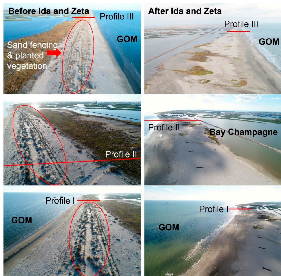
Figure 9. Georeferenced drone images comparing the beach barriers near the three cross-shore profiles before and after Hurricane Ida and Zeta. The red circles mark the sand fences and planted dune vegetation prior to the two hurricanes.
