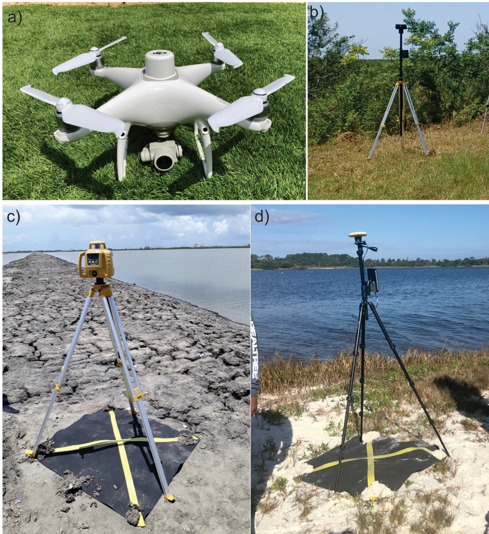
Fig. 1. Essential instruments: (a) Drone Phantom 4 RTK, (b) D-RTK 2 Mobile Station, (c) Electronic Self Leveling Horizontal Rotary Laser, (d) Antenna Trimble Catalyst.
