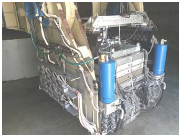
Figure 1. A typical experiment on the 9m centrifuge at UC Davis includes 1500 kg of soil, over 100 sensors, in-flight characterization using cone penetrometers, and multiple simulated earthquake events. Experienced researchers may spend two months building, testing, and excavating such a model. New researchers learn through apprenticeships important centrifuge modeling techniques such as how to place soils, how to calibrate sensors, how to place and log sensors during model construction, how to design a test protocol, and how to manage their test schedule and facility resources, before attempting to lead an experiment.
