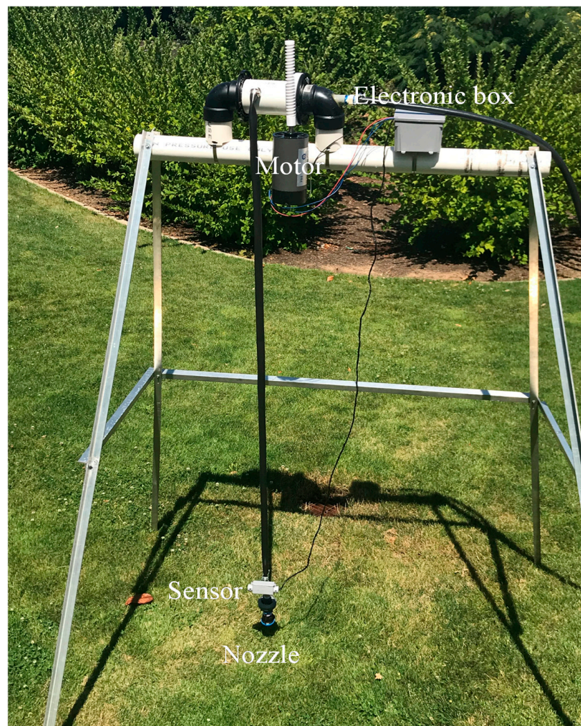
Figure 1. Snapshot for DESA designed and tested with all components to rotate hosepipe back and forth connected with an electronic board assembly with circuits.
