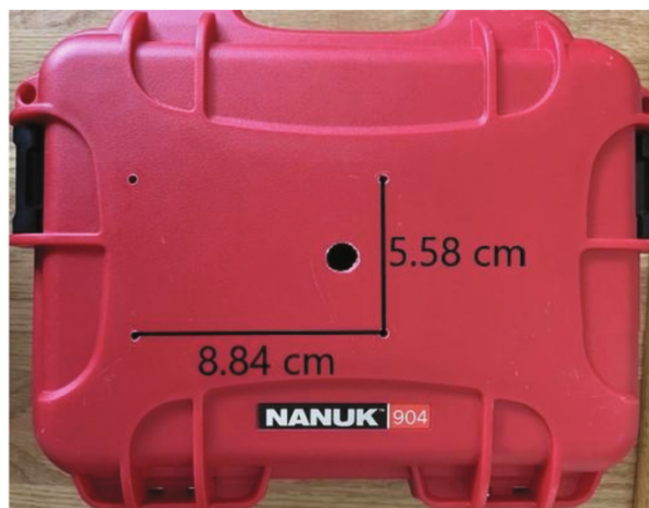
Fig. 9. Sensor cover mounting holes with dimensions and wire through hole.
