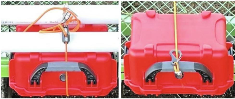
Fig. 15. Case mounted on to PVC frame via rope for proof of concept at 41 cm height (left) and 30 cm height (right).
