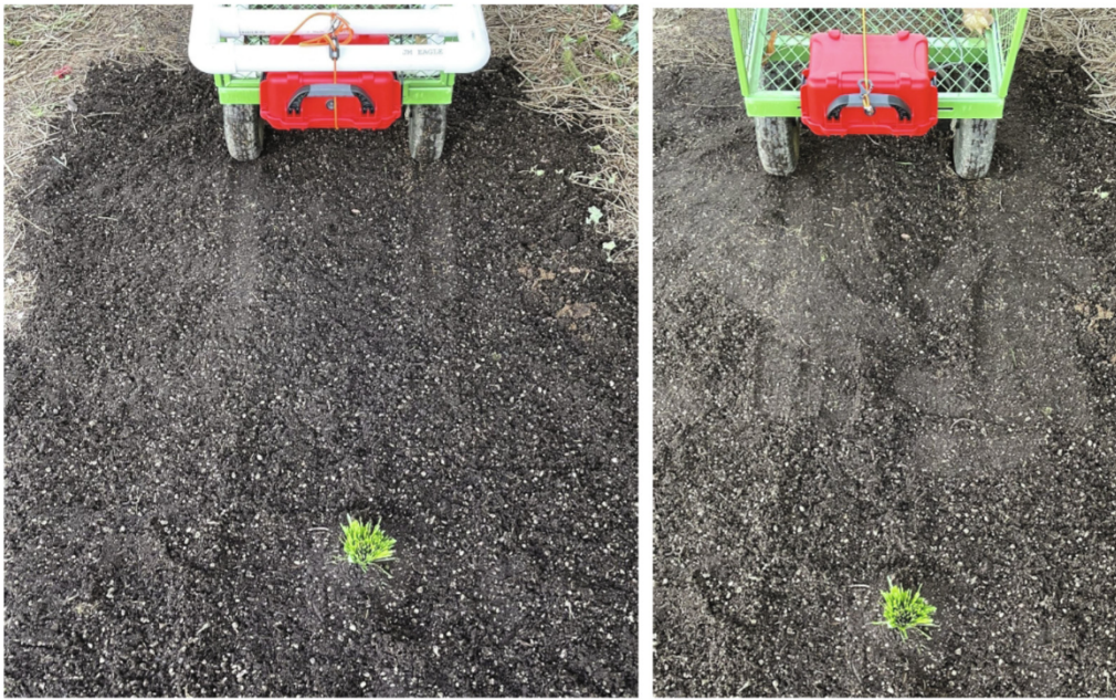
Fig. 17. Weed Warden mounted for testing at 41 cm height, left, and 30 cm height, right.
