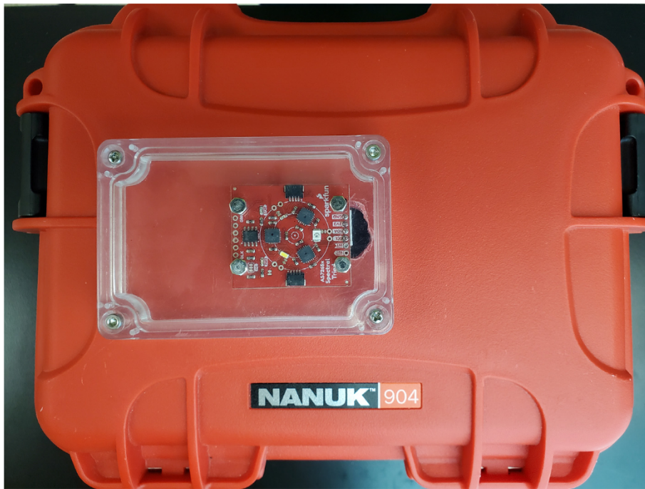
Fig. 12. Sensor cover and sensor mounted on hard case. Note two additional optional screws are shown on triad sensor adjacent to the JST connection.
