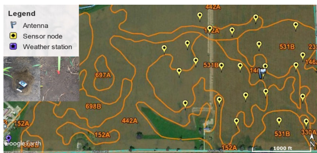
Figure 2. Sensor node locations (yellow pins), base station location (flag), weather station (purple pin), and soil types (orange lines and numbers denote USDA soil type assessment). Inserts show a sensor node deployed in the soil.
