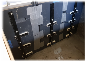
(c) Modified probe array with reduced length of the stainless steel electrodes without insulating covers and grid arrangement as used in the run-out tests
