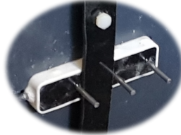
(b) Modified probes using heat-shrink as an insulating cover over the stainless steel electrodes and vertical arrangement as used in Madabhushi et al. (2020)
