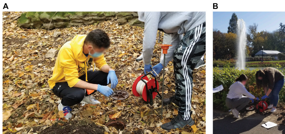
FIGURE 2 | (A, B) Students in general education class ES 1200: Introductory Earth Science Lab used a beep tape to measure depth to water in shallow wells during the pandemic. Masks were required for participation, and laboratory gloves were provided. Photographer: Rowan McLachlan.
